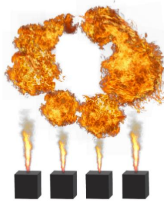
Fig. 1. Schematic illustration of the envisioned setup, where four flame projectors produce a circle of flames
